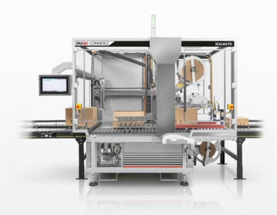
**E-CO Flex SealMatic** is a fully automated case sealer for processing **FEFCO 201 boxes**. It automatically adjusts its mechanical movements according to the case size. SealMatic is equipped with **sustainable water-activated tape technology** to seal cases on top and bottom at high speeds, up to 20 boxes per minute, without the need for operator intervention.
