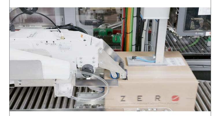
As an optional feature, the E-CO Flex can be equipped with a Print & Apply unit, enabling the seamless placement of a shipping label on the finished case.
