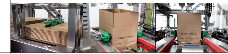
The E-CO Flex boasts the market's widest case magazine, capable of accommodating up to 12 distinct box sizes. This intelligent system efficiently selects the most suitable box size based on the volume of each individual order to be packed.
