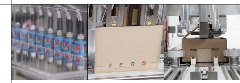
Upon inserting the open-faced case into the closing module, a bank of ultrasonic sensors meticulously measures the remaining void within the box.
