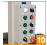
Manual & automatic controls with easy jam clearing
