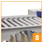
Powered exit conveyor to ensure even small cases exit completely
