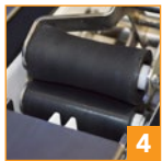
Pneumatic double wipe down of tape legs
